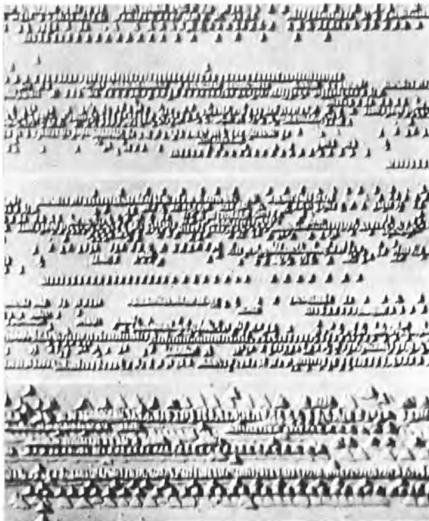
Fig. 10. Etch-pit distribution on the cross-slip surface of an \alpha -copper-aluminum alloy illustrating pileups of positive and negative dislocations in near-edge orientation on adjacent glide planes. Magnification \sim 1750\times . (Mitchell et al. 78 Reproduced by permission of the National Research Council of Canada from the Canadian Journal of Physics .)
