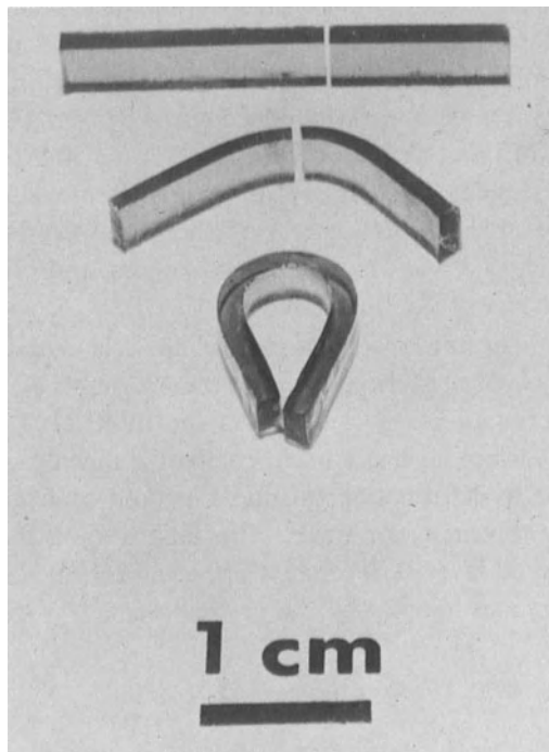
Fig. 36. Illustrating Joffe's effect with irradiated potassium chloride crystals. Upper crystal deformed in air; middle crystal immersed in water for 60 sec, dried, and then deformed in air; lower crystal deformed under water. (After Westwood. 186 )
