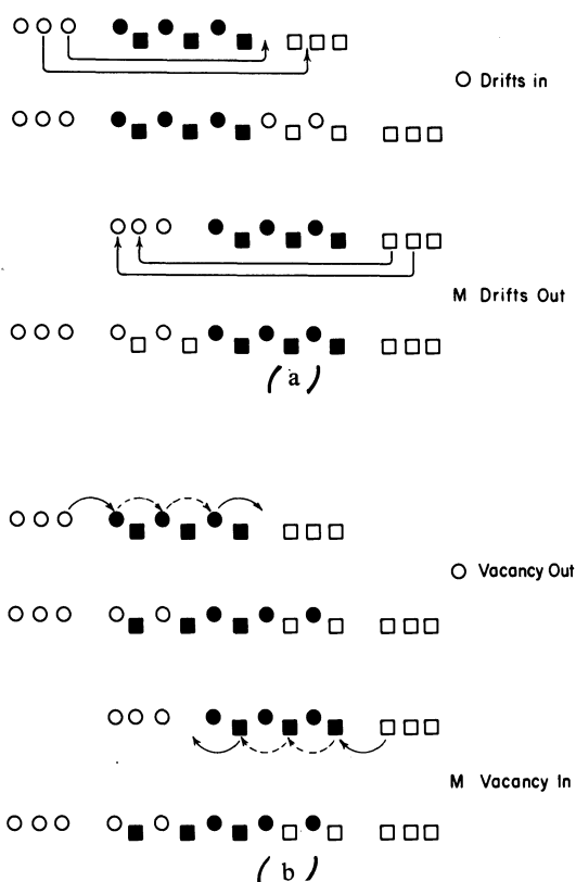
Fig. 27. Symbolic representation of the basic ion-transport models. a) Direct movement. b) Propagation. ○) Oxygen; ●) labeled oxygen; □) metal; ■) labeled metal. (After Amsel and Samuel. 272 )
